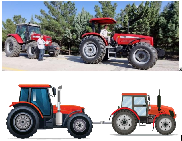
Fig 3. The drawbar traction force tests with ballast (a) and schematic of connected exhaust pipe to the exhaust manifold of the load tractor (b)
