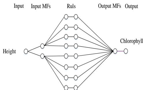
Fig 2. The structure of Neuro-Fuzzy system (ANFIS)
